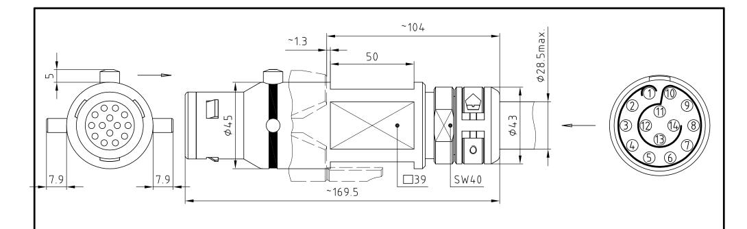
Outer shell : Stainless steel (AISI304) : Stainless steel (AISI416) Latch sleeve : Stainless steel (AISI304) Inner shell : Stainless steel (AISI304) Front ring Collet nut + clamps + screw : Stainless steel (AISI304) : PEEK Insulator : Brass (UNS C38500) Male contact Clip
